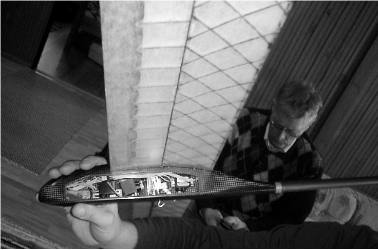
Fig. 4 (top) Flaps have been lowered, conferring the airfoil an ample undercamber of 7.8% at 47% chord,
